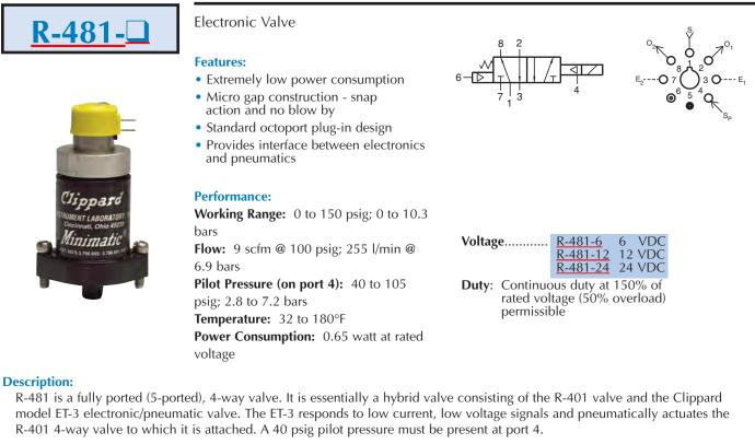
model ET-3 electronic/pneumatic valve. The ET-3 responds to low current, low voltage signals and pneumatically actuates the R-401 4-way valve to which it is attached. A 40 psig pilot pressure must be present at port 4.
